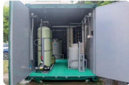
20 tons \ day two level seawater desalination equipment Singapore
